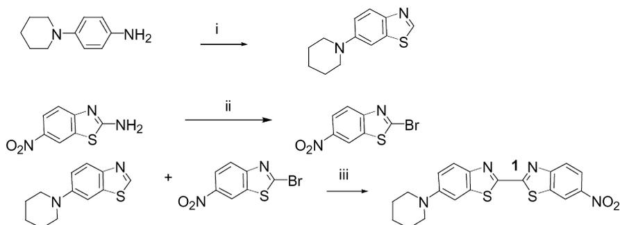
**Scheme 1.** Reagents and conditions. (i)  $\text{Na}_2\text{S}_2\text{O}_3 \cdot 5\text{H}_2\text{O}$ ,  $\text{K}_2\text{Cr}_2\text{O}_7$ , AcOH, 0 °C, 8 h, r.t. overnight, 34%. (ii)  $\text{NaNO}_2$ , CuBr, HBr 48%. (iii) Bu–Li, anh.  $\text{ZnCl}_2$ , CuI.
