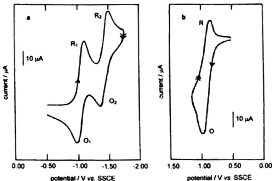
**Figure 1.** Cyclic voltammograms for the (a) reduction and (b) oxidation of a 1 mM **1** solution in  $\text{CH}_2\text{Cl}_2$  with 0.1 M tetrabutylammonium perchlorate at  $200 \text{ mV s}^{-1}$  and at 25 °C on a  $0.093 \text{ cm}^2$  Pt electrode. Initial potential: (a)  $-0.50$  V, (b)  $0.50$  V. Reversal potential: (a)  $-1.800$  V, (b)  $1.200$  V.
